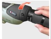
Insert the eyepiece and twist clockwise until the eyepiece clicks in to the locked position.
