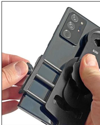
2. Set the height of the phone clamp (C) to securely hold your smartphone model in the adapter by turning the clamp adjustment knob (E), turning clockwise lowers the clamp, turning anti-clockwise raises the clamp.
