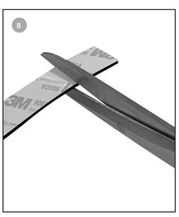
**8.** When combining rubber adjustment strips, for a neat and more stable fixing, you should trim down the length of the inner strips to avoid overlapping. This will help keep a more central alignment.
