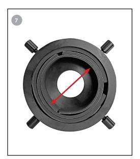
7. Remember - if you are using an eyepiece with a narrow diameter, you can combine the rubber adjustment strips to reduce the diameter of the adapter ring.
