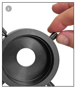
**2.** As standard, the SMARTOSCOPE UR-4 eyepiece ring is designed for larger eyepieces. Turning the securing screws clockwise engages the inner compression ring which is used to secure the adapter ring on to your eyepiece and for reducing the diameter of the outer ring if your eyepiece is smaller than the standard adapter diameter.
