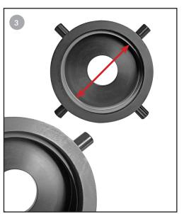
3. When the compression ring is engaged - the diameter is reduced, it also protects your eyepiece from contact with the adjustment screws and helps to ensure a stable secure fit. When reducing the size of the SMARTOSCOPE UR-4 adaptering by using the compression ring - be sure to turn all 4 adjustment screws equally to ensure centralised alignment with your eyepiece.
