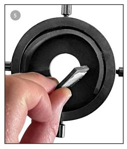
**5.** Before removing the adhesive strip cover - check which strip or combined strips is the best combination to securely push over your eyepiece. The fit should be firm but should allow for pushing on and removal of the adapter ring without force.
